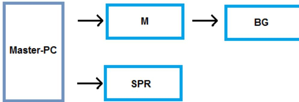
The machine M and the machine BG are cascaded, in the sense that BG is supplied by M with data. The control system ("Master PC") sends data in parallel to M and SPR.
