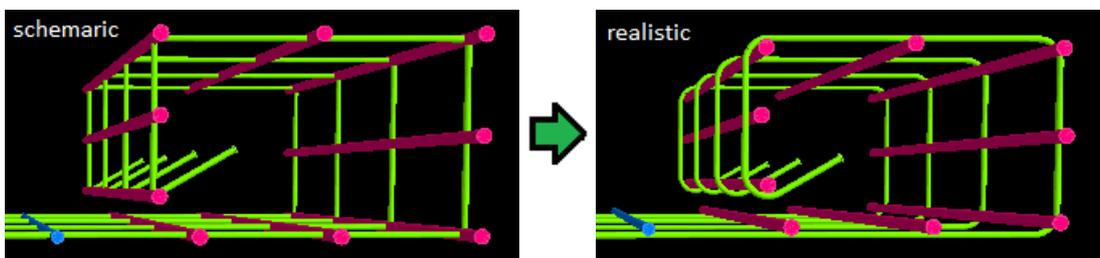
For bending angles of up to 90°, the bending shape simply is rather more "angular" than in reality. For bending angles above 90°, however, the outer shape will be shown distorted.
