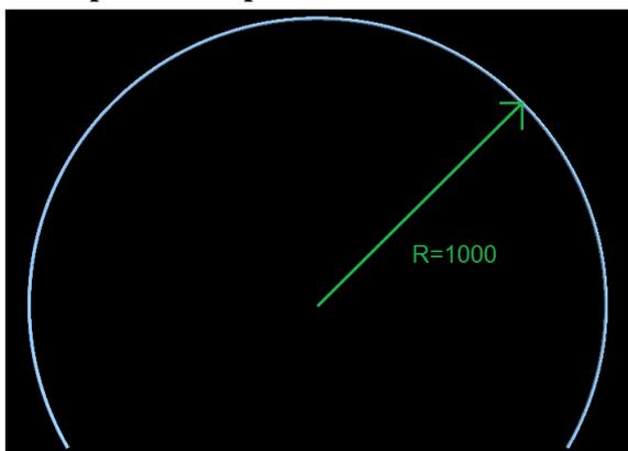
An arc with an arc radius of 1,000 mm (core dimension) and an angle of 240° will be represented via two segments:
