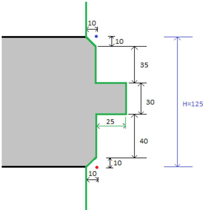
The following examples describes the important cases of "bottom chamfer", "top chamfer" and "no chamfer":
