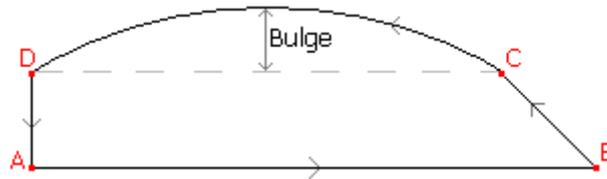
This figure shows a *Shape* with 4 vertices. A, B and D are to have a  $Bulge=0$ , whereas the value of *Bulge* for C is positive; with a negative value of *Bulge*, the arc would be curved inwards, i.e. the sign of *Bulge* indicates the arc orientation class.
