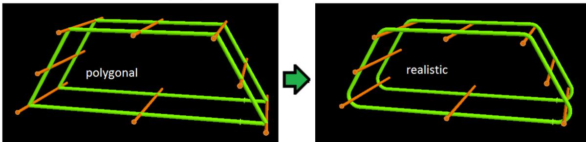
For bending up to 90°, the representations of *schematic* and *polygonal* tally with each other. However, both representations differ when it comes to acute bends: the *polygonal* representation remains true to the real shape of the rebar, whereas the *schematic* representation modifies the outer proportions<sup>35</sup>.
