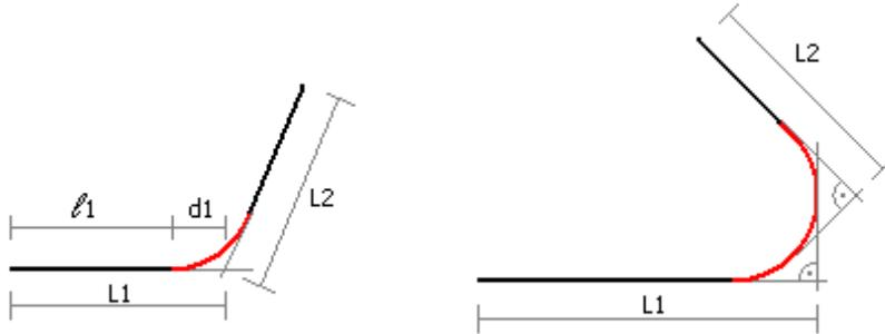
For angles not larger than  $90^\circ$ ,  $R$  will have *no* effect on the bending shape, but merely results in the corners being rounded. The basic shape will then be given by the theoretical lengths. For bending angles beyond  $90^\circ$ ,  $R$  will have a direct effect on the overall dimensions.
